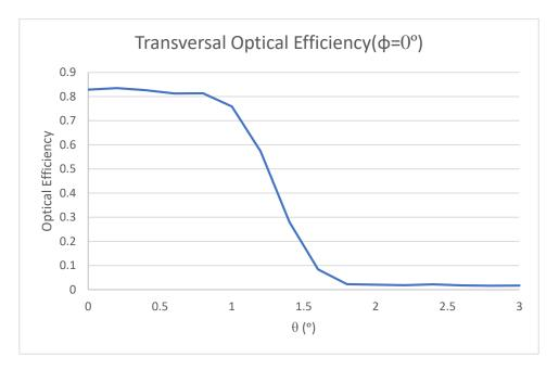
Fig. 18. Transversal efficiency curve of the collector.
